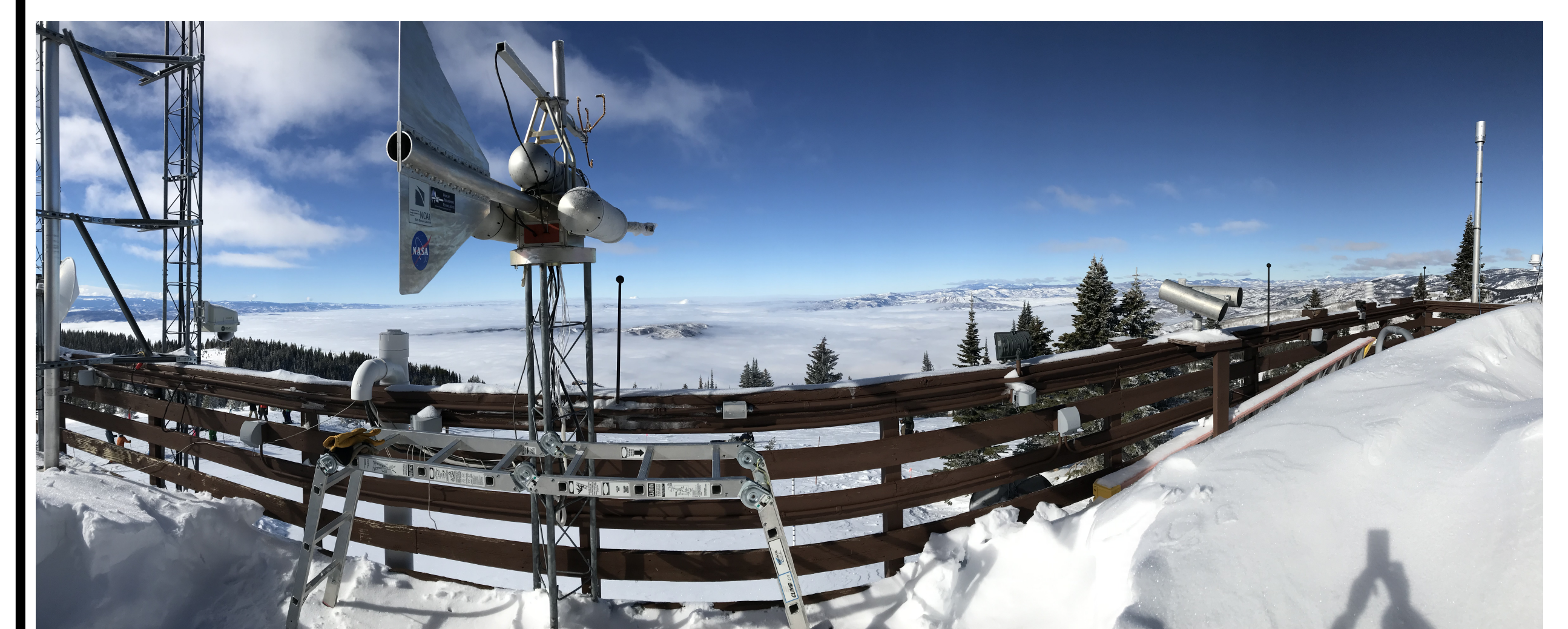
Gannet, Maria and Ian spent January 2019 at Storm Peak Laboratory making aerosol and cloud microphysical measurement to validate the MIT Spider inlet
